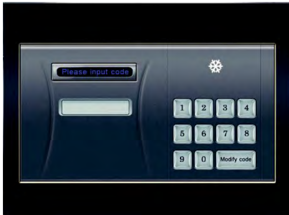
(Fig 1) Input default password: “000000” (Pass if use IC card control) to enter interface as (Fig 2) shows.
